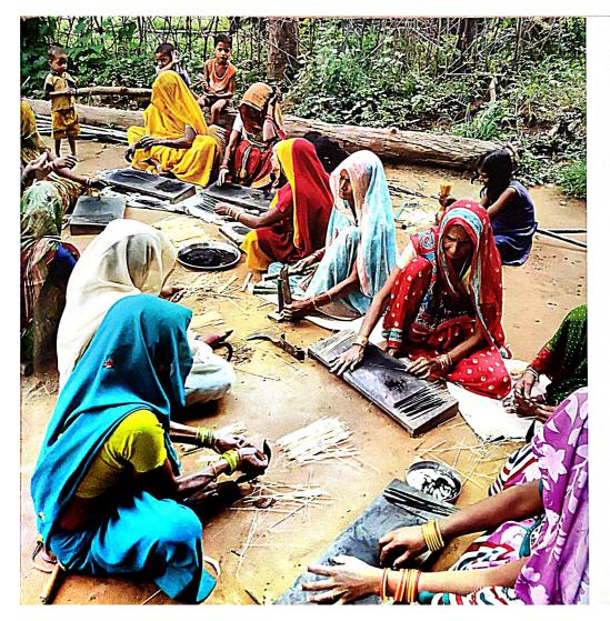
The production process of Agarbatti essentially entails four stages: (1) production of bambos sticks for the central core of the Agarbatti; (2) production and preparation of charcoal and Giggat powder; (3) preparation of incense paste (Masala) and its application onto the bambos stick to produce the batti; and (4) scenting, or application of perfume, to produce a good quality Agarbatti, followed by packaging. The value addition between these stages is nearly exponential.
